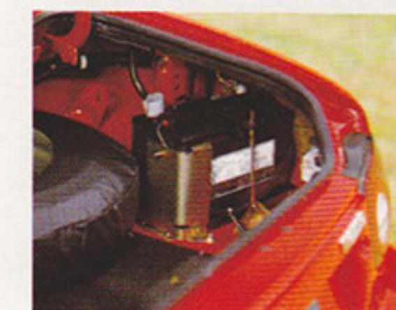
In the interest of balance and weight saving, the battery found a home in a corner of the boot. It's compact, weighs only 9kg yet provides 32 ampere-hours of capacity.
