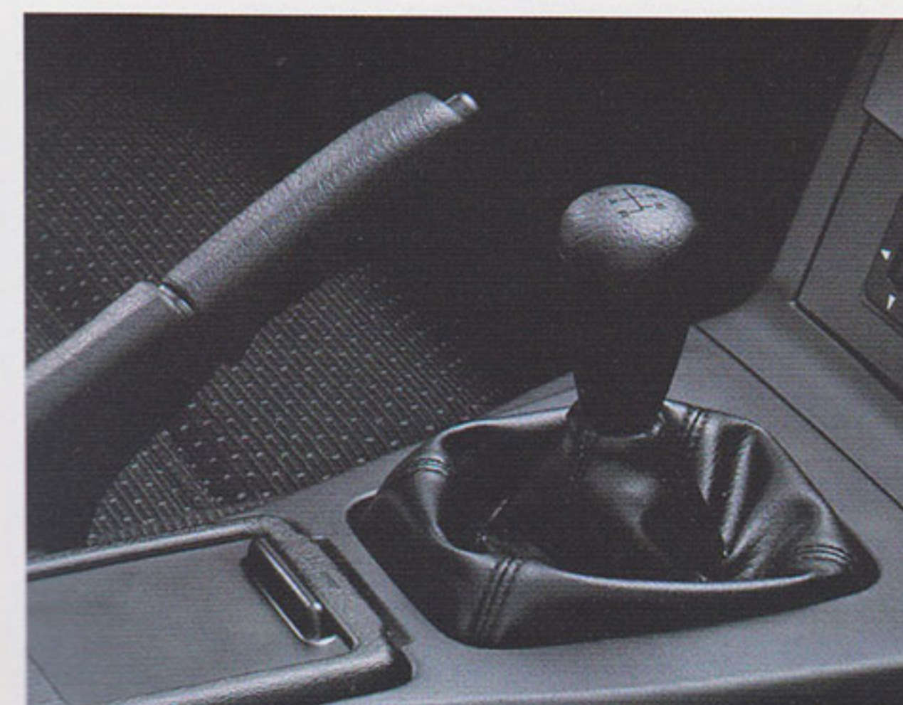
The short-throw gear stick is coupled to a close ratio gearbox for precise changes.
