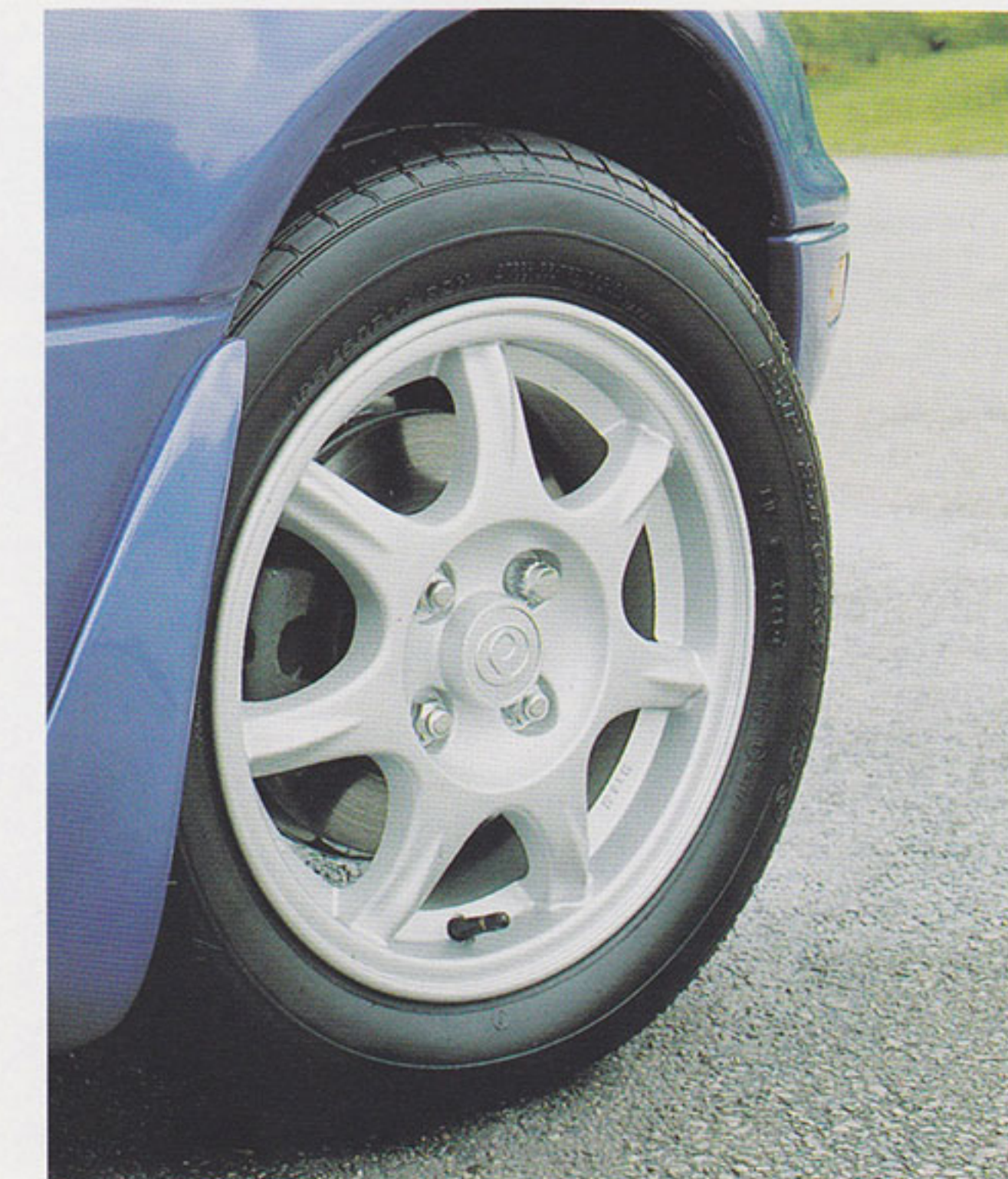
New style alloy wheels 14 x 6.0JJ are standard equipment on the new Mazda MX-5 1.8iS model.
