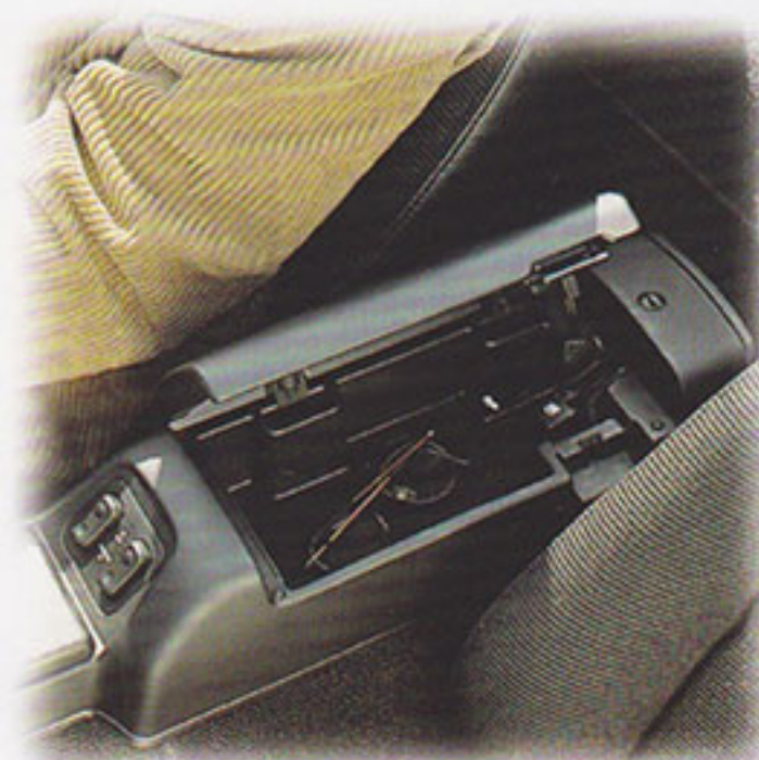
Lockable central pocket houses remote petrol lid opener and boot release for 1.8 models (1.6i model remote petrol lid opener only)
