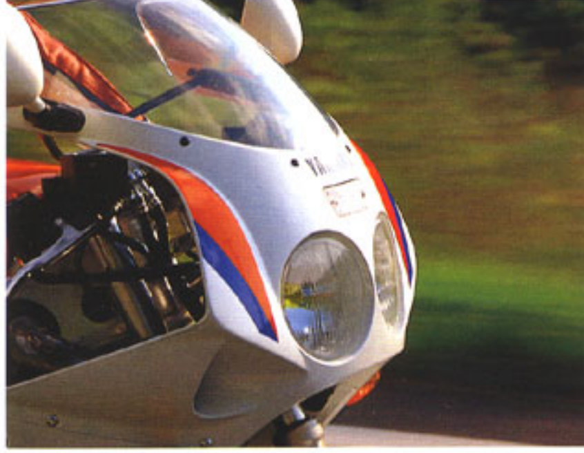
New fairing with FAI system A new fairing has flush-fitting headlight lens and a greater rake to the upper cowl for better air-penetration. The FAI (Fresh Air Intake) system in the fairing sides routes cool, dense air to the carburetor airbox for better cylinder breathing and more performance.
