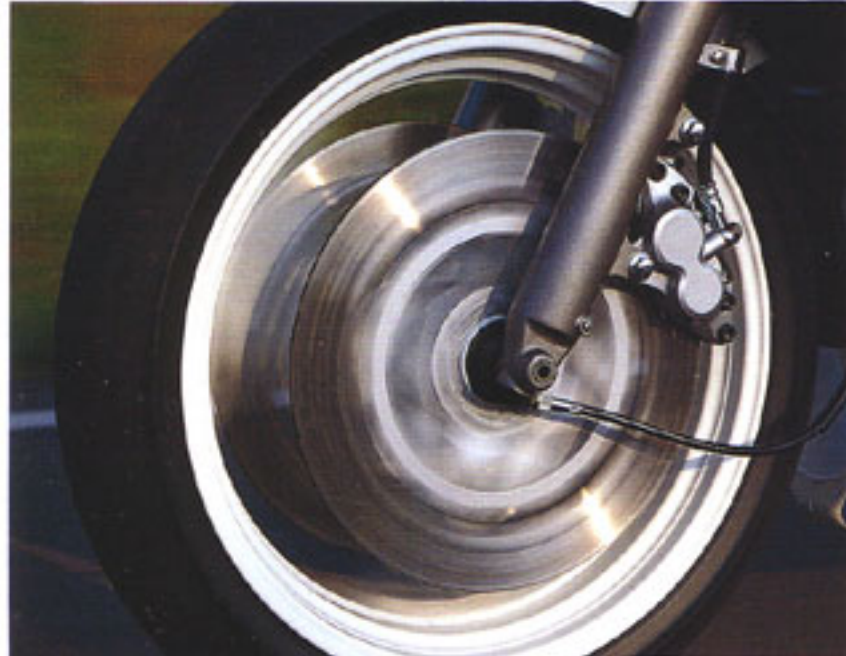
Massive forks and new front brake Front fork stanchion diameter is increased from 41mm to 43mm for increased rigidity. Unequal piston sizes (larger diameter for the top pair) in the new-design hydraulic calipers provide the rider more "feel" when using the dual 287mm disc brakes.
