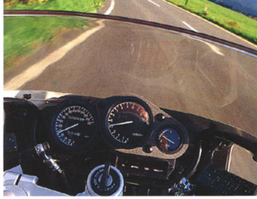
Redesigned instrument panel The redesigned instrument panel is more compact, with smaller meters and the tachometer more prominently-positioned for quick reference. An electrically-operated fuel switch allows the rider to change to reserve supply with minimum effort.
