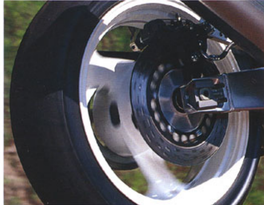
Deltabox swinging arm and adjustable shock New Deltabox swinging arm is constructed in light alloy and triangulated for maximum lateral rigidity. The Monocross rear shock absorber stroke is increased by new linkage arrangements for improved shock action. The damper is adjustable for spring pre-load and damping rate.
