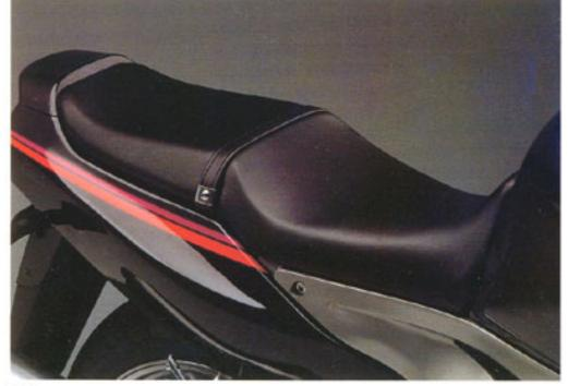
Contoured seat permits maximum rider body movement for increased controllability. Its low 775mm height keeps weight near the ground for optimum centre of gravity and allows the rider to sit in the machine for less drag. Quickly-detachable cover reveals pillion seat for passenger transportation.
