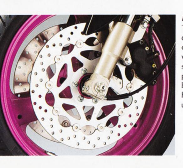
Two large-diameter front disc brakes operated by opposing 4-piston calipers work in tandem with a single rear disc to provide powerful, responsive braking. All the brake discs have been drilled to reduce unsprung weight.
