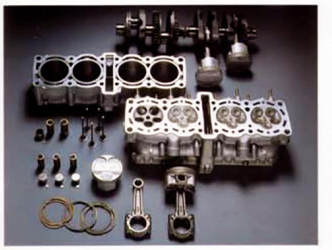
One of the most significant performanceboosting features on the FZR is our 5-valve head design. Featuring 3 inlet valves and 2 larger diameter exhaust valves, this race-developed system achieves an excellent balance between intake and exhaust processes for superior low to mid-range power.
