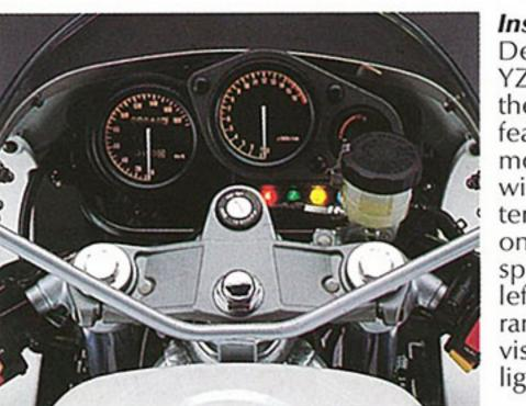
Developed from our YZF400 factory racer, features a centrally-mounted tachometer speedometer on the
