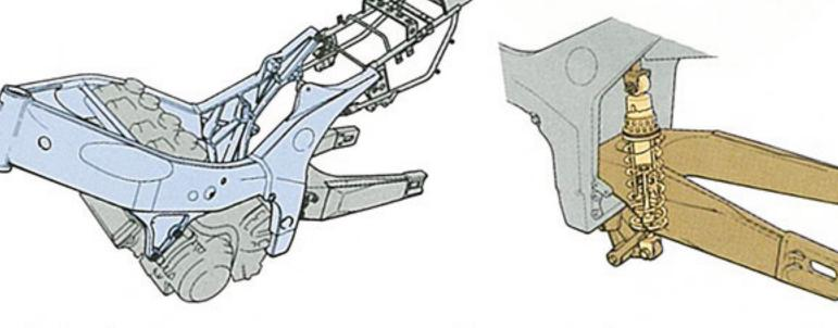
Another spin-off from our factory racing programme is the aluminium Deltabox frame. Using the FZR400RR and extremely light, giving sharp handling.
