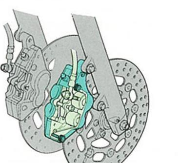
powerful 4-pot calipers ensure progressive and controllable braking power. A span-adjustable lever offers a choice of 4 positions, while further YZF influence is underlined by the separate fluid reservoir.
