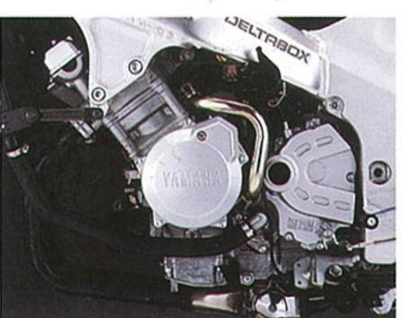
cylinder engine features narrow-angle valves, straight inlet tracts and compact combustion chambers for optimum distribution and low
