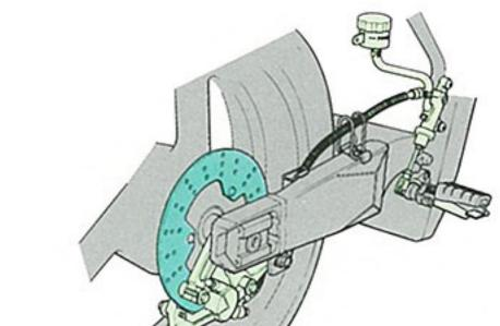
Monocross rear suspension system uses a 9-step preload-adjustable gas/oil shock and lightweight Deltabox
