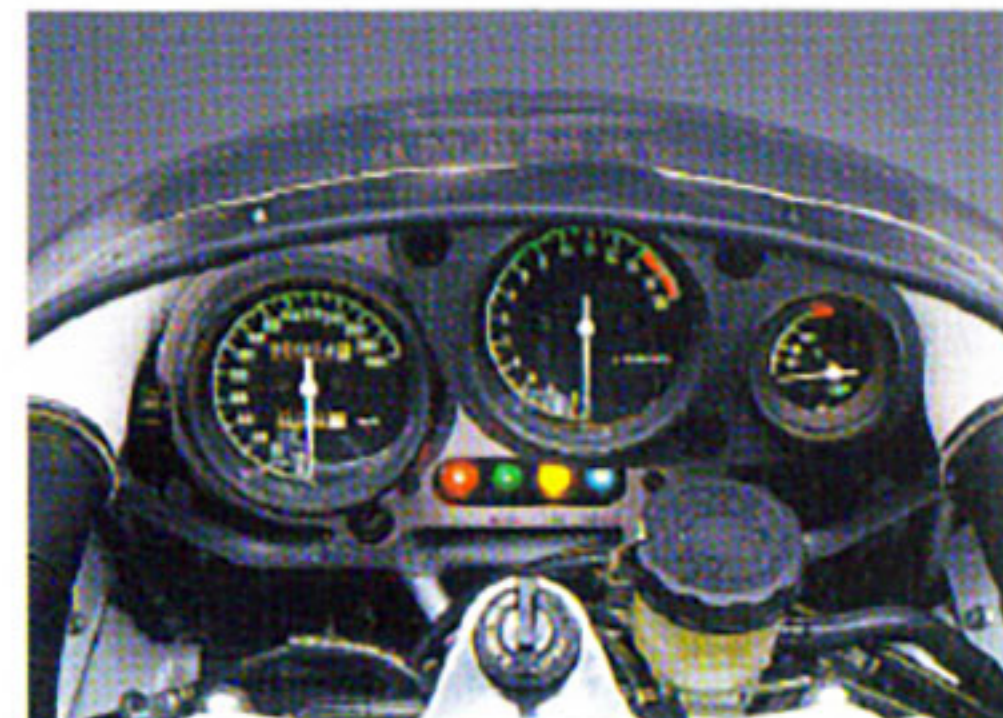
Instrument panel features centrally mounted electronic tachometer, water temperature gauge and easy to read speedometer for at a glance information. Oil, neutral, turn and high beam warning lights complete the neat and compact display.
