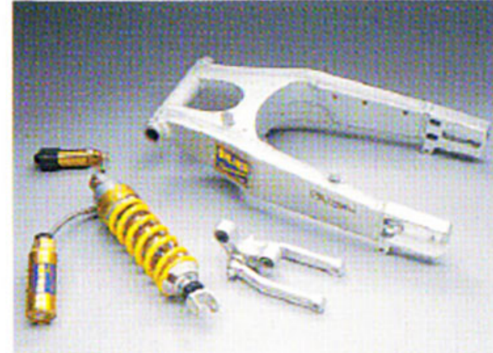
Fabricated lightweight aluminium Deltabox swinging arm keeps unsprung weight low and resists lateral flex forces. Race perfected Öhlins shock absorber and rising rate linkages ensure the rear wheel stays hard against the track surface even under flat out acceleration.
