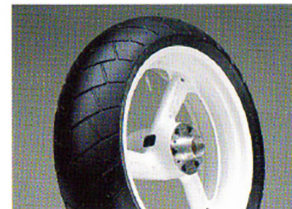
Lightweight alloy triple hollow spoke wheels are taken straight from our Grand Prix winning YZR racers. For 1990 they are fitted with new wider and lower profile Michelin Hi-Sport radial tyres to give even better traction.
