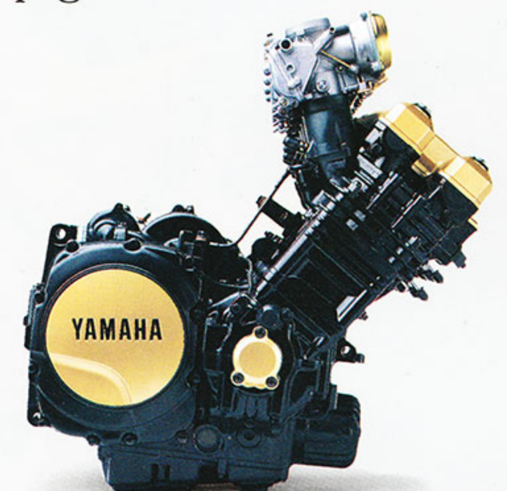
The Genesis engine's 45° cylinder angle makes room for special downdraft CV carburetors and gives the mixture a straighter, more efficient path into the cylinders.
